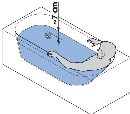
The tub is provided with an electronic sensor which prevents the pump from starting if the water level is lower than the minimum. Therefore, if the pump does not start when the button (B) pressed and you hear a long beep, add water and press the button again.
