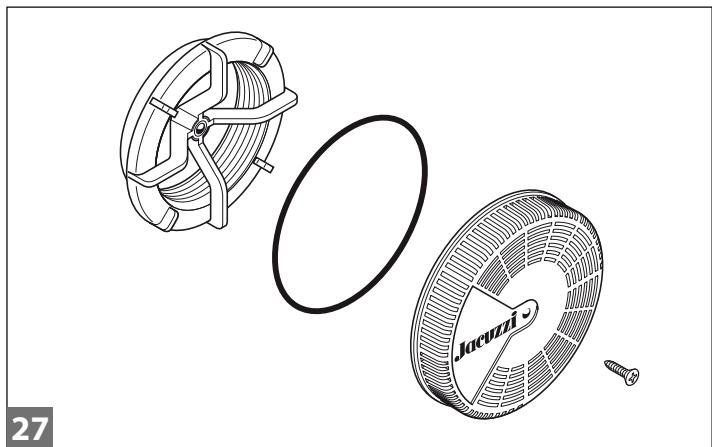
■ (☞ 27) Remove the screw and cover (be careful not to release the clip of the inside flap).
