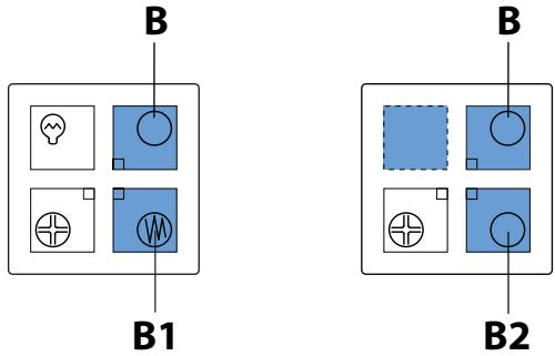
**B**) hydromassage cycle on/off button (pump 1)
