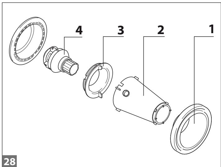
■ (☞ 28) Remove the flange cover (1) by levering under the edge with a wide flat tipped screwdriver.
