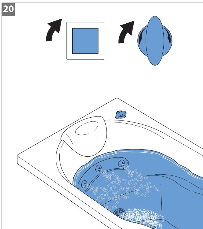
the flow of water to the backrest nozzles or to the large nozzle underneath (☞ 19-20).
